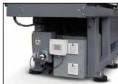
*You can now fit hydraulic power units directly under the ECSXIII, thanks to the machine's redesigned, space-saving frame (power units not included). Its streamlined design also allows easy access to electrical panels and components.*
