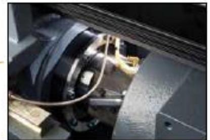
*The ECSXIII uses an advance load cell which ensures accurate control of injection pressure. In combination with the V70 controller, this load cell achieves Scientific Molding over the balance of the mold without the use of internal transducers.*
