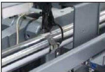
Strain gauge adjusts tonnage automatically and on the fly during the cycle. This ensures accurate tonnage at all times.
