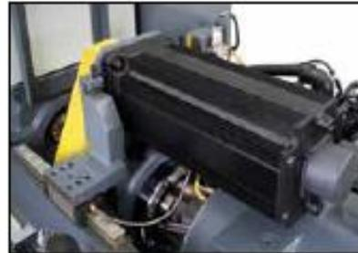
*The heavy weight on the injection unit is supported on linear guides, greatly reducing the drag of injection and backpressure.*
